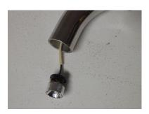
5. Push the new LED assembly into the front of the end cap making sure the wires exit through the back side of the end cap. Connect the quick disconnect fittings to the new assembly.
