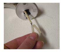
4. Push the LED wires until the LED assembly exits the front of the end cap. Pull the LED completely out of the end cap.
